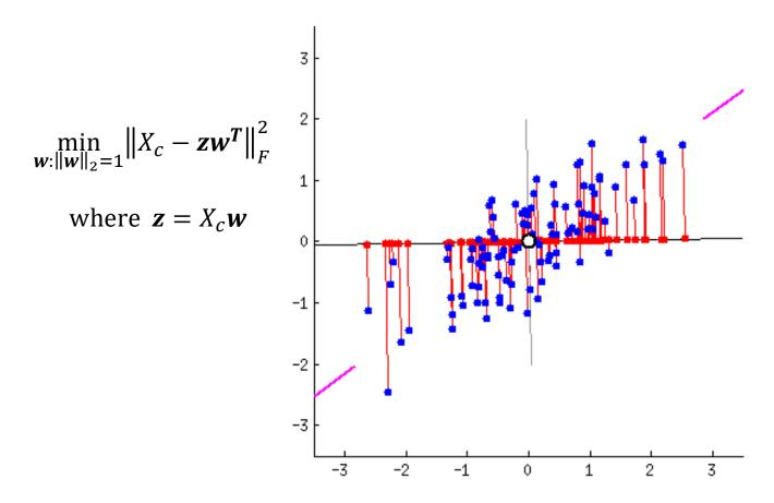
2D to 1D projection: Red lines show the projection error onto 1D lines. PCA finds the line that has the smallest projection error (in this example, when it aligns with the purple).
